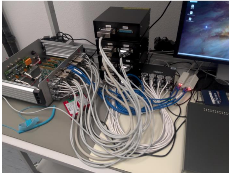
Fig. 3. SDVF with OBC Hardware in the Loop and Interface Cards
