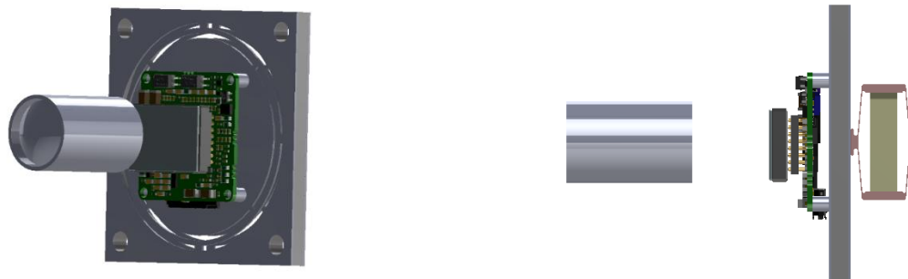
Figure 5: Front (left) and side (right) views of the focusing mechanisms with the detector board. The piezo actuator (yellow) is to be glued to the amplifier (red) after a precise deformation is imposed on the latter. This ensures the correct preload is applied to the actuator. The external case is removed for clarity.
