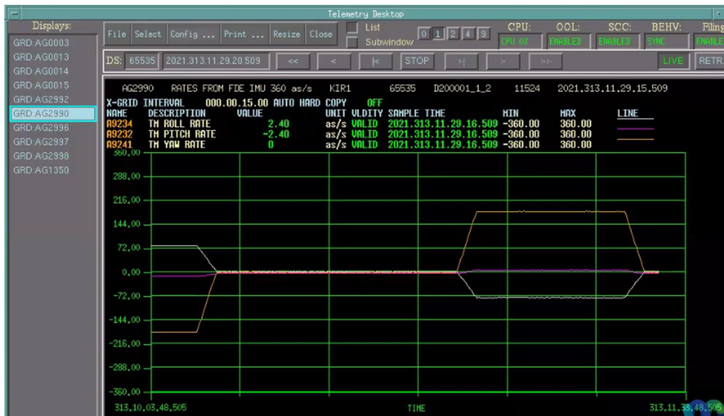
Figure 7 Gyro-slew, plot of angular rate TM during GSL commissioning, Nov 2021
