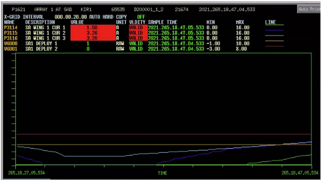
Figure 10 Solar array currents from the 3 panels of wing 1, at start of manual speed commanding. The TM display shows red warnings, indicating array outputs below the normal range.
