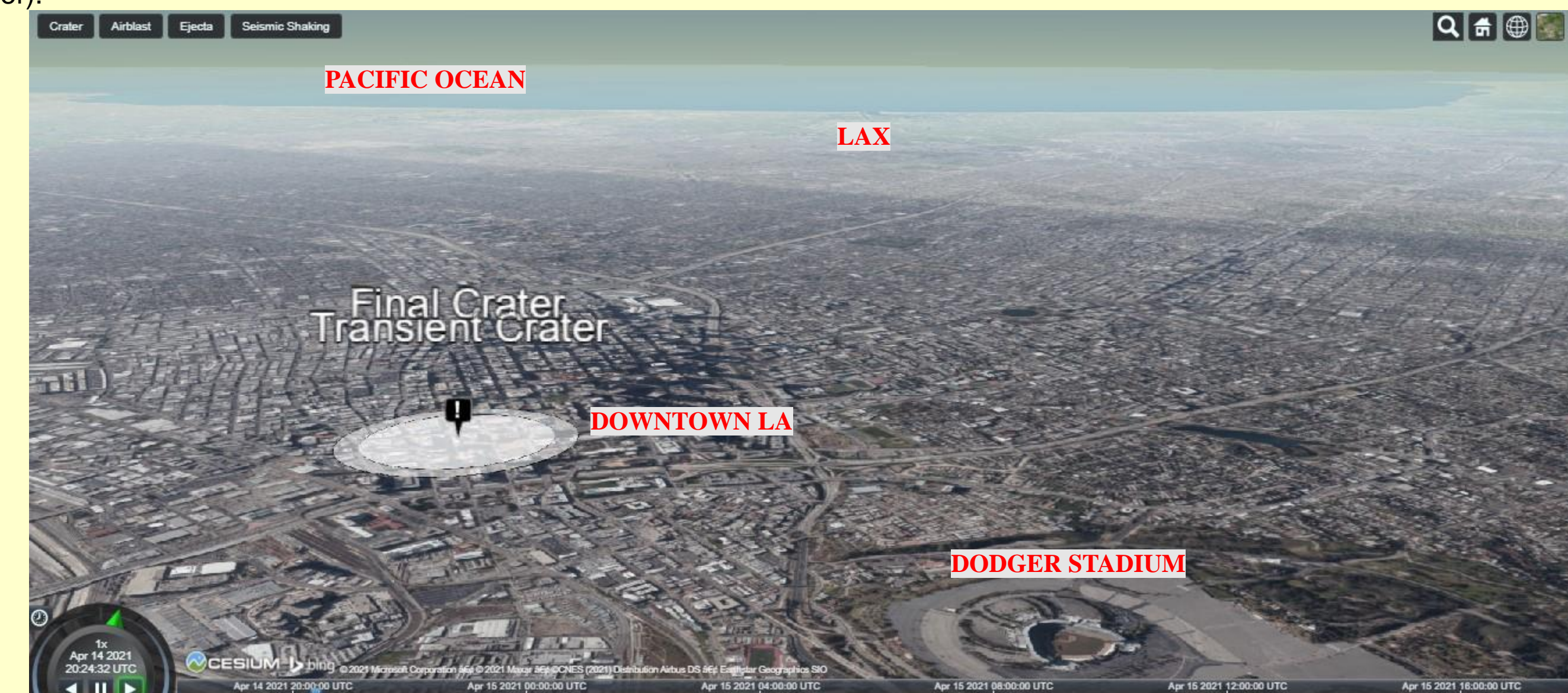
Figure 4. Impact crater of diameter 0.825 km and depth of 176 m formed from a 30-m diameter iron object with a density of 8000 kg/m 3 traveling at 12 km/s in Downtown Los Angeles.
