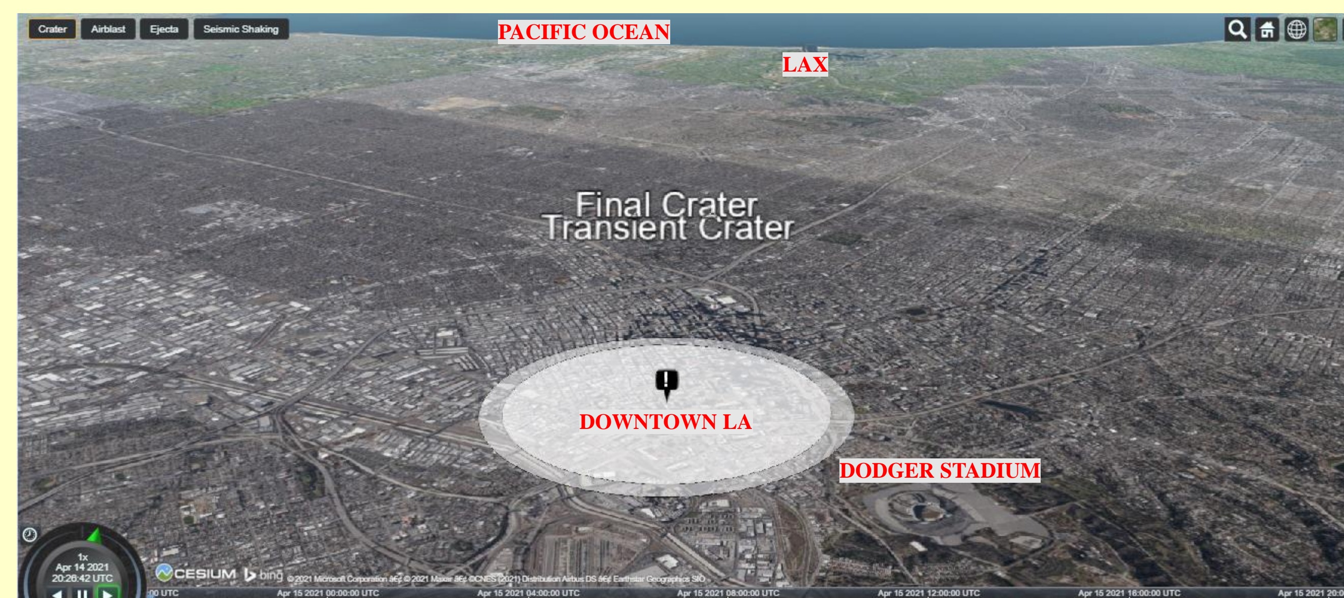
Figure 5. Impact crater of diameter 2.97 km and depth of 411 m formed from a 300-m diameter porous rock object with a density of 1,500 kg/m 3 traveling at 12 km/s in Downtown Los Angeles.
