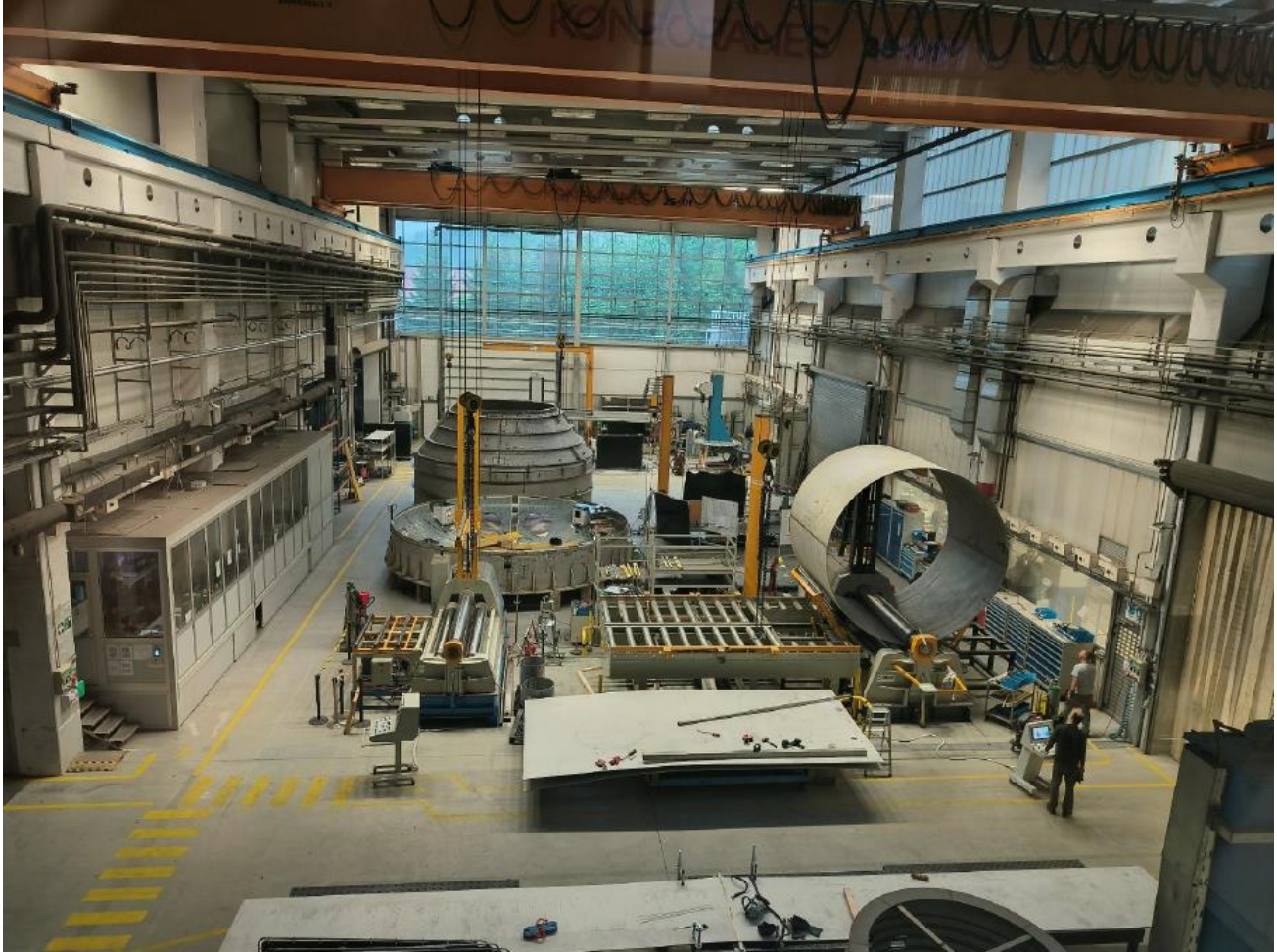
Figure 8. Vacuum Vessel under preparation at the Brinox facility
