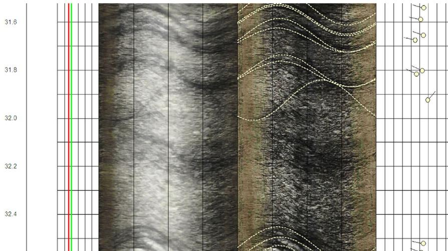
Fig. 10. A typical test section with multiple pre-existing fractures. Scanning before test (left) and after test (right).
