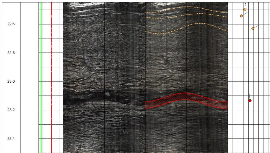
Fig. 9. A condition with large open joint making it impossible to build up pressure. Scanning before test (left) and after test (right).
