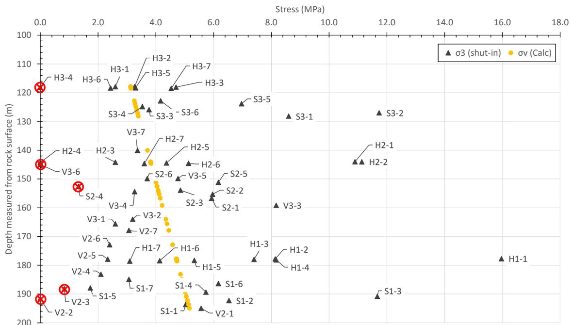
Fig. 5 Estimated shut in pressures based on pressure curve obtained inside test sections, plotted versus the depth from surface. The vertical stresses were calculated based on unit weight of the rock and overburden. A sequential number is added to the drillhole name to indicate the sequence of the test.
