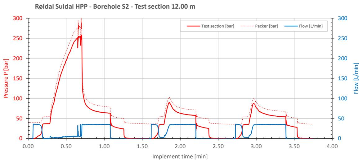
Fig. 6. A typical hydraulic test that can be considered to be a HF test, which is characterised by significantly higher  $P_{max}$  in the first test cycle than  $P_{max}$  in the subsequent test cycles.
