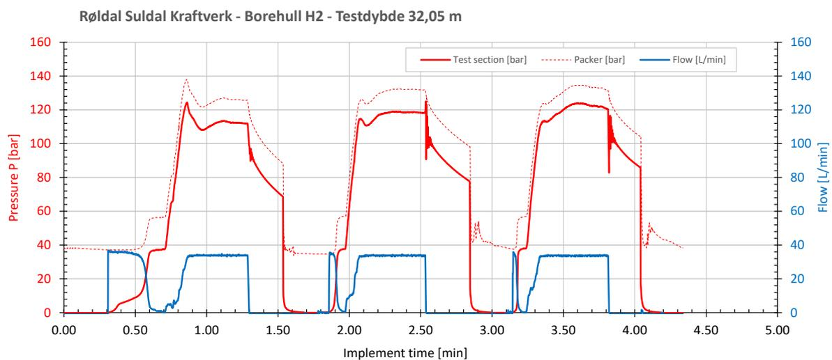
Fig. 7. A typical hydraulic test that can be considered to be a HTPF test, which is characterised by a similar  $P_{max}$  in all test cycles.
