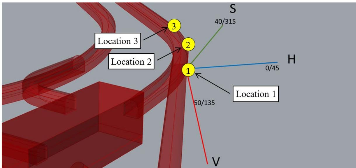
Fig. 4 Layout of the drillholes at the end of the access tunnel.
