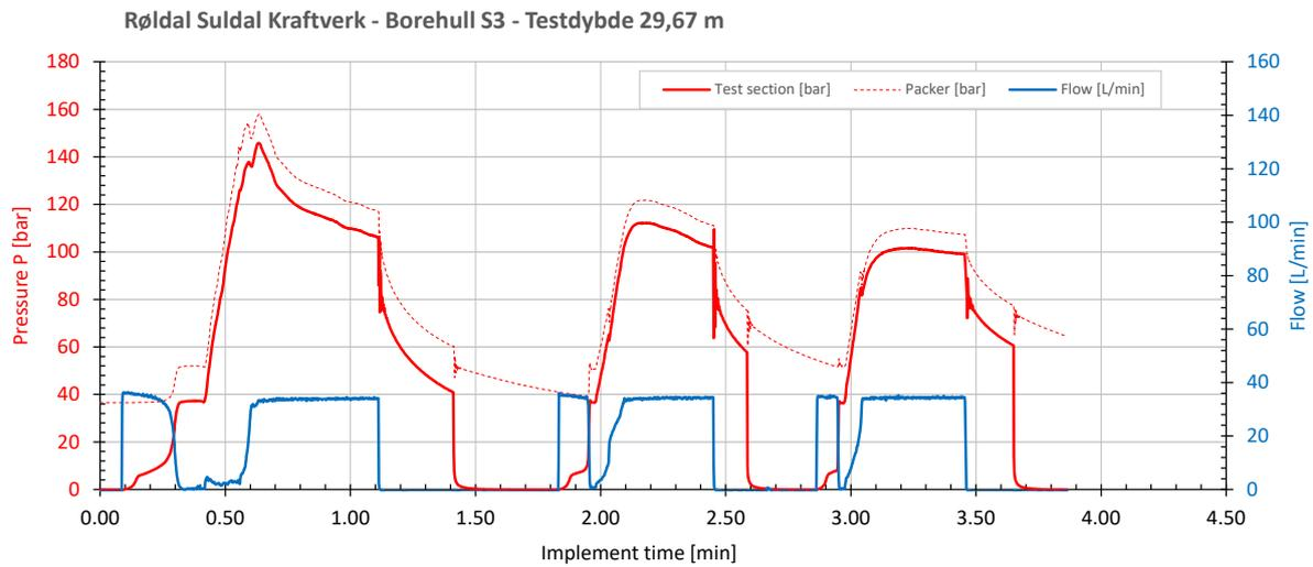
Fig. 8 A typical hydraulic test that cannot be clearly classified as a HF or HTPF test.
