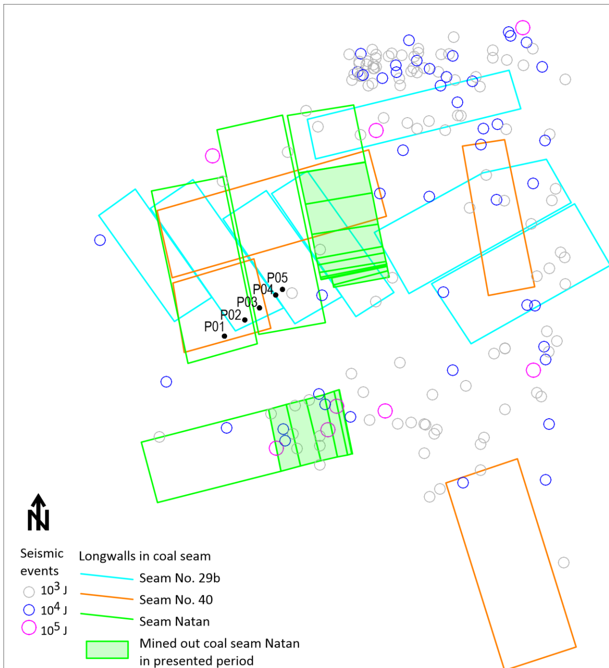
Fig. 5 Registered induced seismicity during mining of longwalls in Natan coal seam in period from January 2023 to April 2024
