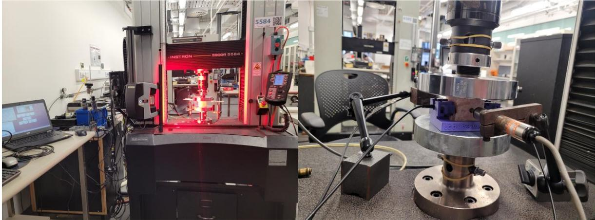
Fig. 1: (a) Instron Machine for inducing damage and UCS testing, (b) Ultrasonic sensors and LVDTs attached to the sample.
