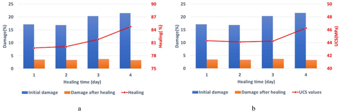
Fig. 7 a. Healing percentage versus time for rock salt under high humidity and temperature conditions, b. UCS values for healed samples subjected to high humidity and temperature at different time intervals.
