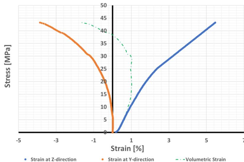
Fig. 2. Uniaxial compressive strength (UCS) test results for rock salt samples.
