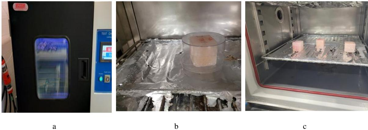
Fig. 5 a) Environmental chamber used for testing, b) Specimen covered with glass dishes to block moisture, c) Samples placed inside the environmental chamber.
