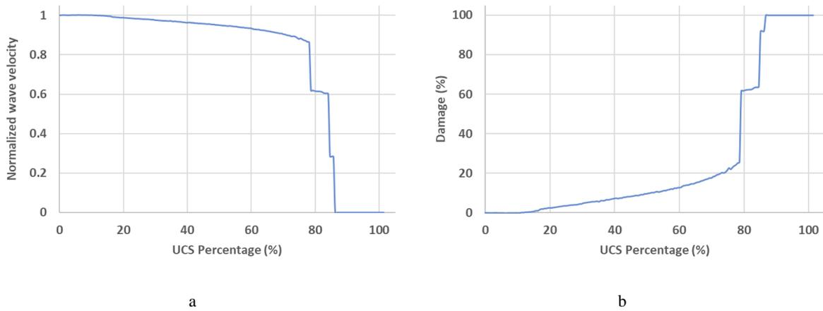
Fig. 3 a) Normalized wave velocity versus loading, b) Damage calculated based on ultrasonic measurements versus loading.
