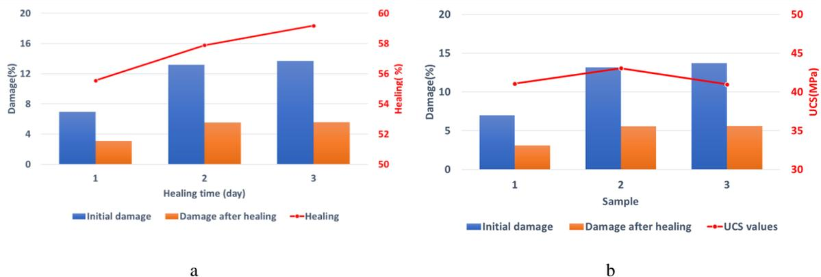
Fig. 6. a. Healing percentage versus time for rock salt under high humidity and temperature conditions, b. UCS values for healed samples subjected to high humidity and temperature at different time intervals.
