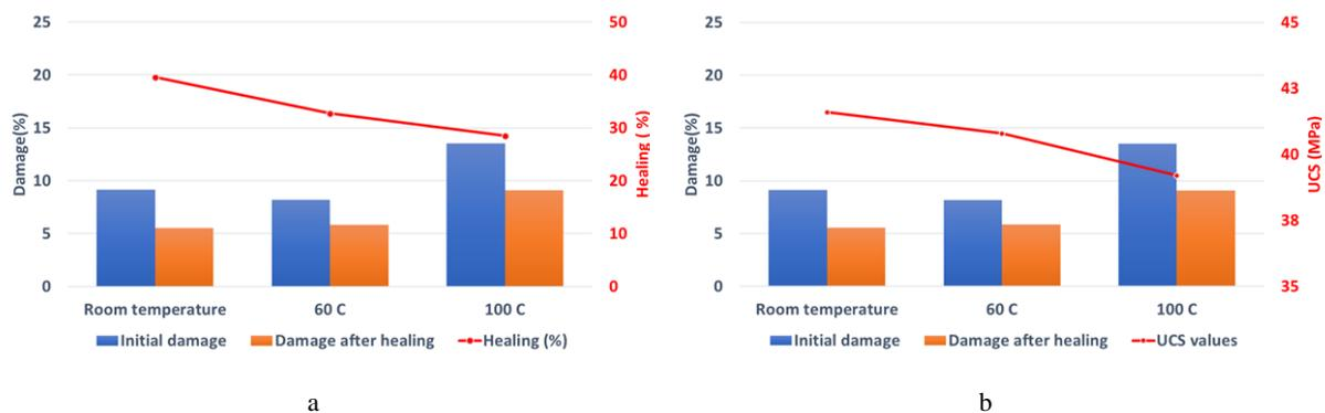
Fig. 4 a) Healing percentage for rock salt under different conditions at 50% UCS, and b) UCS values correspond to 50% UCS recovery tests.
