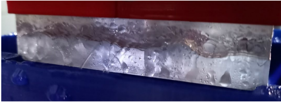
Fig. 12 Jet-like outflow, characteristic of high stresses and pressures
