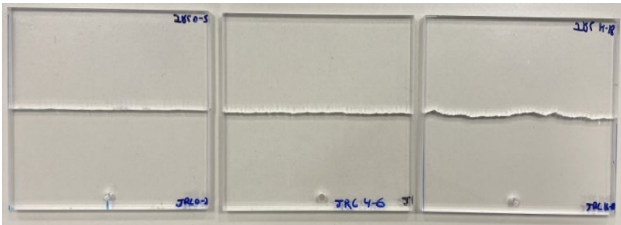
Fig. 1 Plates with JRC of 0-2, 4-6 and 16-18 respectively
