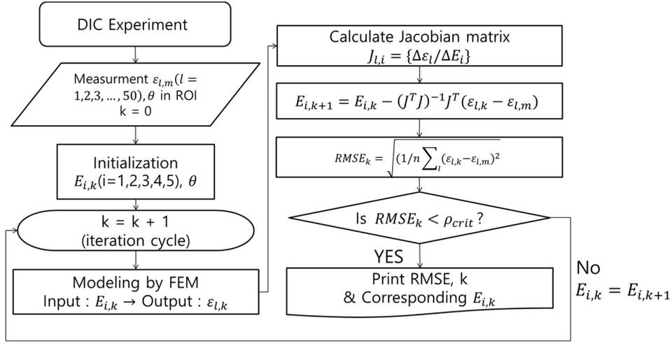
Fig. 2. Flow chart of Gauss–Newton method (m : measured, k : iteration number,  $E_i$  : i-th elastic constant,  $\varepsilon_l$  : l-th strain value)
