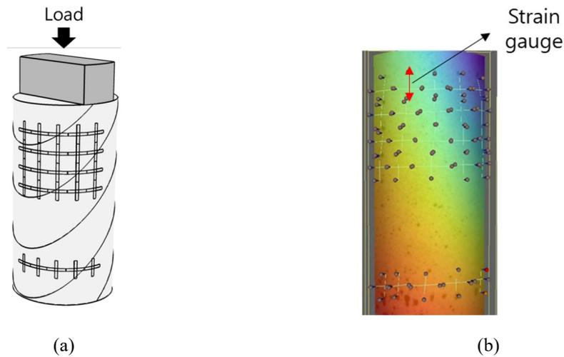
Fig 1. (a) Schematic diagram of strip load test and (b) axial displacement image measured by DIC, in which the region of interest is divided into fifty virtual strain gauges, each with a gauge length of 1 cm
