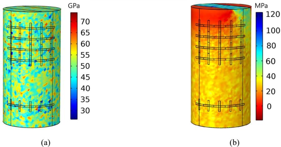
Fig. 3. Distribution of elastic constant E in cylindrical heterogeneous transversely isotropic specimen (b) and stress distribution when the bedding angle is  $45^{\circ}$
