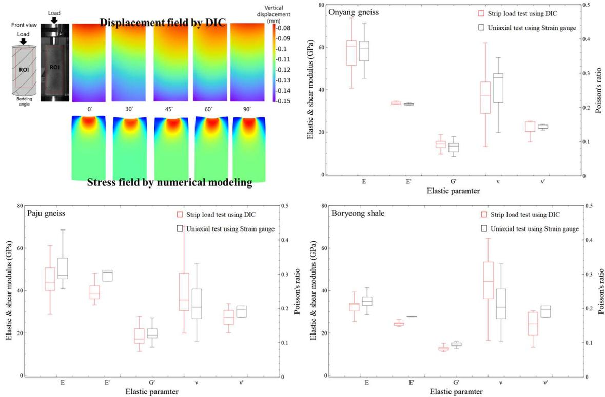
Fig. 5. Displacement field measured by DIC in transversely isotropic rock and the corresponding axial stress distribution at the same angles obtained through numerical analysis and boxplot of the five elastic constants determined from stress-strain values measured by DIC and strain gauges under uniaxial compression for Onyang gneiss, Paju gneiss, and Boryeong shale
