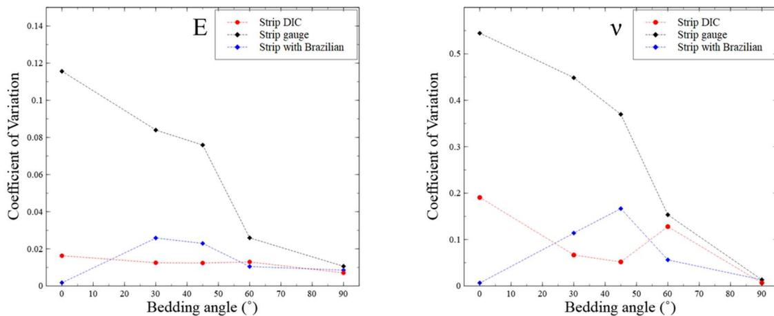
Fig. 4. Variation of the coefficients of variation for E and  $\nu$  at different bedding angles under strip load, measured by Digital Image Correlation (DIC), strain gauges, and with the addition of Brazilian tests.
