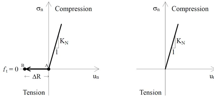
Fig. 3 Normal stress vs relative normal displacement for the shield (left) and for the lining (right).
