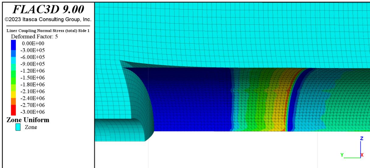
Fig. 10 FLAC3D model ( $\Delta R=10\text{cm}$ ) deformed mesh and normal stress contours on the springs
