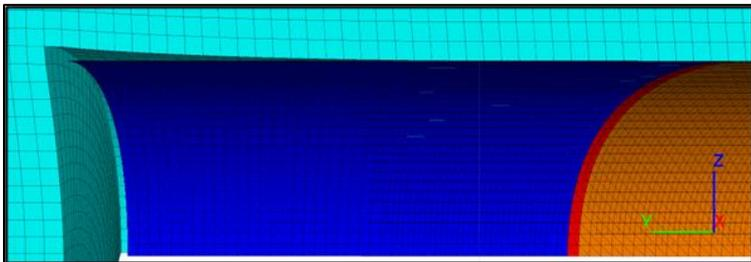
Fig. 8 Restoring of shield stiffness and installation of a segmental lining slice
