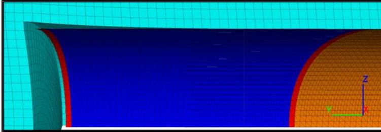
Fig. 7 Initialization of the overcut through application of a radial displacement to the structural nodes
