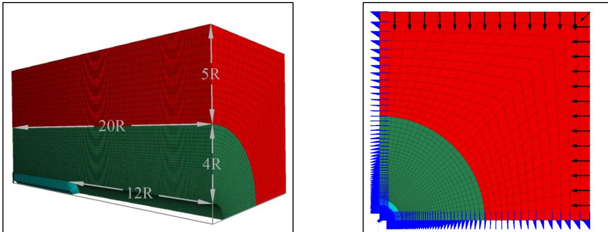
Fig. 2 Model details and mesh.
