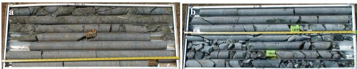
Fig. 2 Example drill core from the study area indicating variation of rockmass quality and structures. a) shear zone. b) fracture zone
