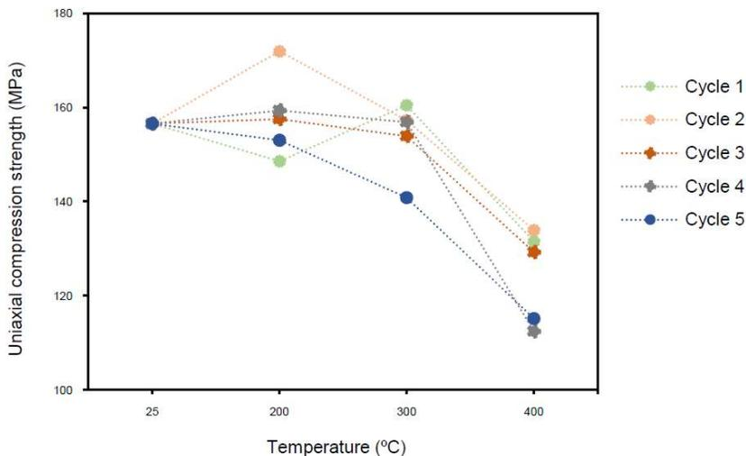
Fig. 5 Uniaxial compressive strength in response to temperature increase and thermal cycling.
