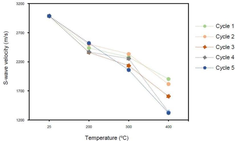
Fig. 3 S-wave velocity variation as a function of temperature and number of thermal cycles.
