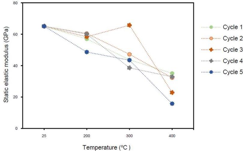
Fig. 6 Behavior of the static elastic modulus as a function of temperature increase and number of thermal cycles.
