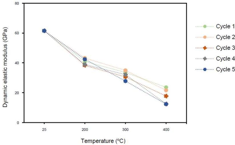
Fig. 4 Dynamic elastic modulus as a function of temperature increase and number of thermal cycles.
