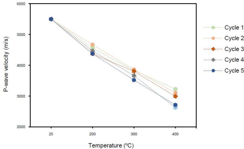
Fig. 2 P-wave velocity variation as a function of temperature and number of thermal cycles.
