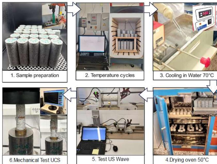
Fig. 1 Experimental workflow and laboratory equipment used in research.
