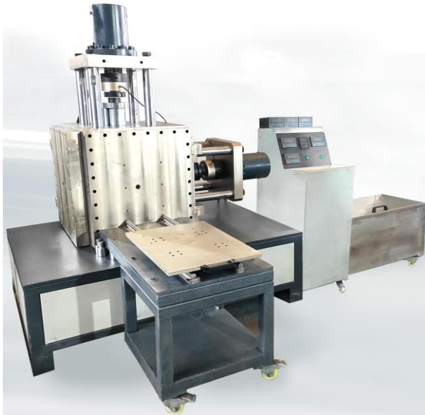
Fig. 2 Physical Test System for Multi-field Coupling Effects newly developed by Tsinghua University.
