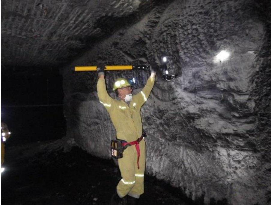
Fig 3 Side wall scanning conducted using Frequency Modulated Continuous Wave radar device.
