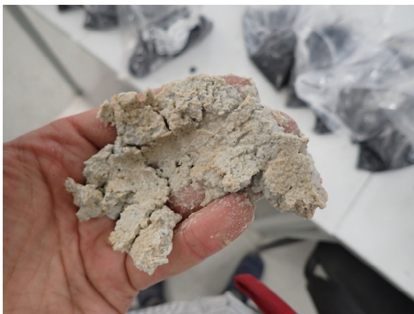
Fig. 3: Difficult assessment of fine-grained cuttings.
