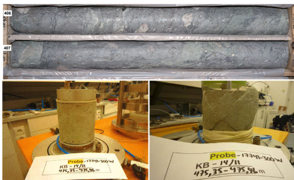
Fig. 2: Rock mechanics investigations on fault material.
