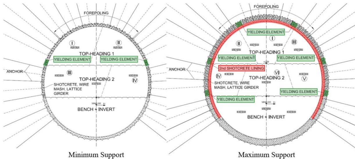
Fig. 3 Schematic illustration of different support types for the Grassberg-Schlagl fault system (left: low deformation; right: high deformation)
