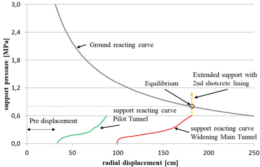
Fig. 8 Ground reaction curve and support reaction curve for a ductile support system with pilot tunnel and additional shotcrete layer
