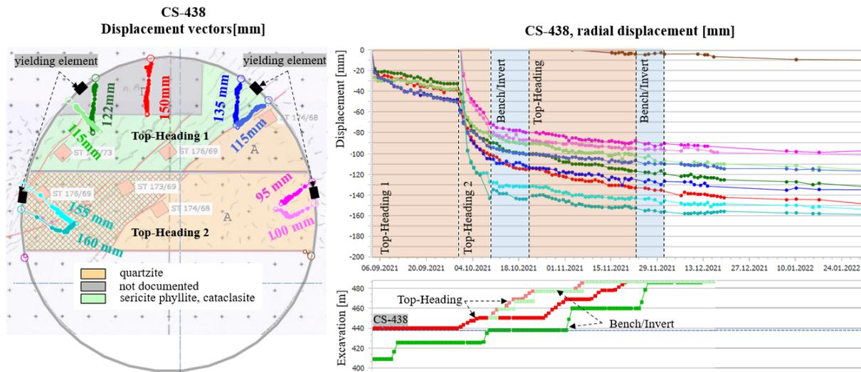
Fig. 4 CS-438, Displacement vectors in the cross section overlaid with the documented geology (left) and time-displacement graph for the radial displacements (right)
