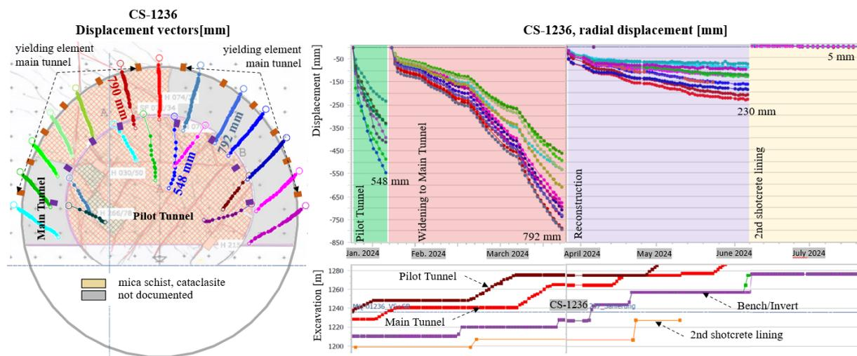
Fig. 9 CS-1236, displacement vectors in the cross section overlaid with the documented geology (left) and time-displacement graph for the radial displacements (right)
