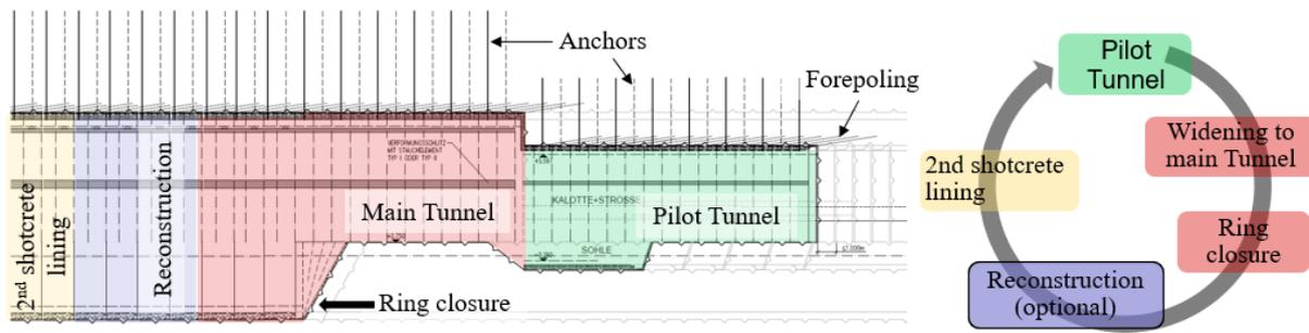
Fig. 6 Construction sequence with pilot tunnel and second shotcrete lining
