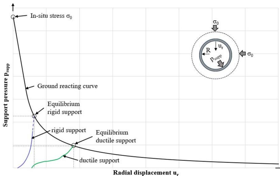
Fig. 2 Ground reaction curve and support reaction curve for a rigid and ductile support system
