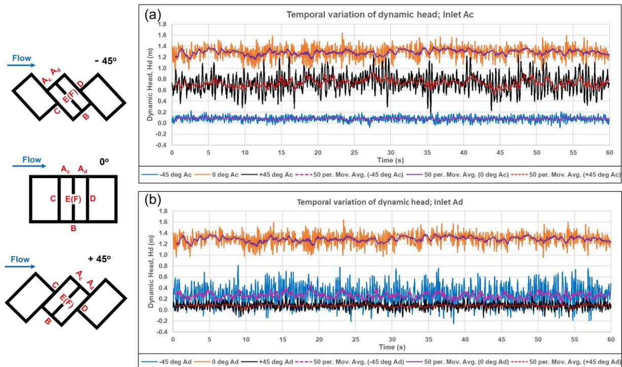
Fig. 3 Temporal variation of dynamic head on the top of the block for different joint orientations: (a) Water inlet Ac; (b) Water inlet Ad.
