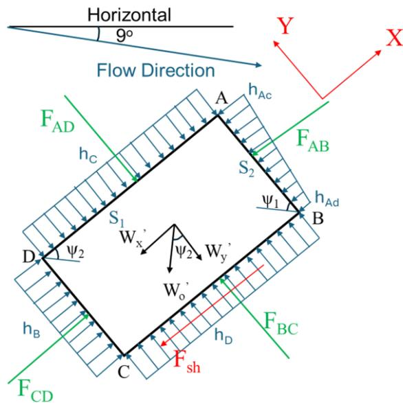
Fig. 6 Pressure distribution around the blocks aligned towards the direction of flow (Considering unit length along the lateral direction).
