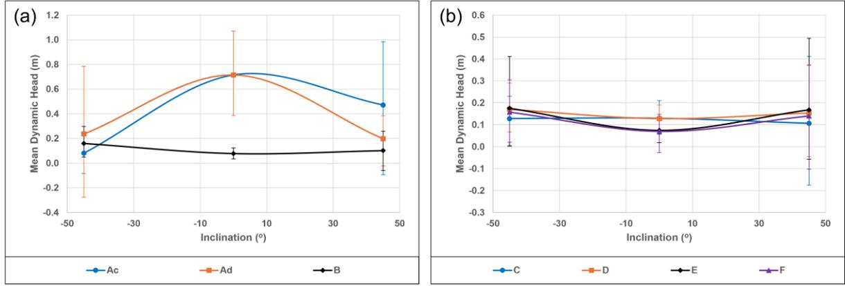
Fig. 4 Variation of dynamic head with joint orientation at different joint inlets: (a) Top and bottom of the block; (b) Lateral sides of the block.
