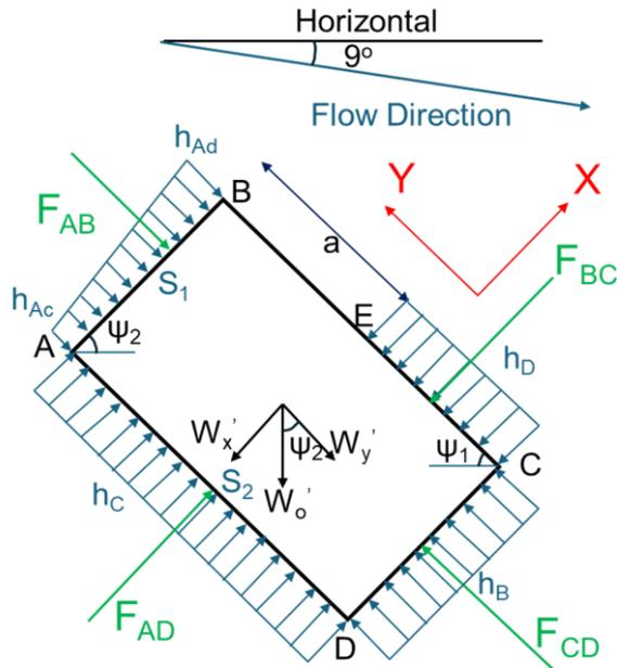
Fig. 5 Pressure distribution around the blocks aligned against the direction of flow (Considering unit length along the lateral direction).
