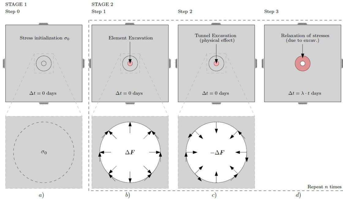
Fig. 2 Boundary conditions applied at each step of the simulation to model the spalling phenomenon. Additionally, a detailed representation of the excavation process employing the strategy of applying equivalent forces.
