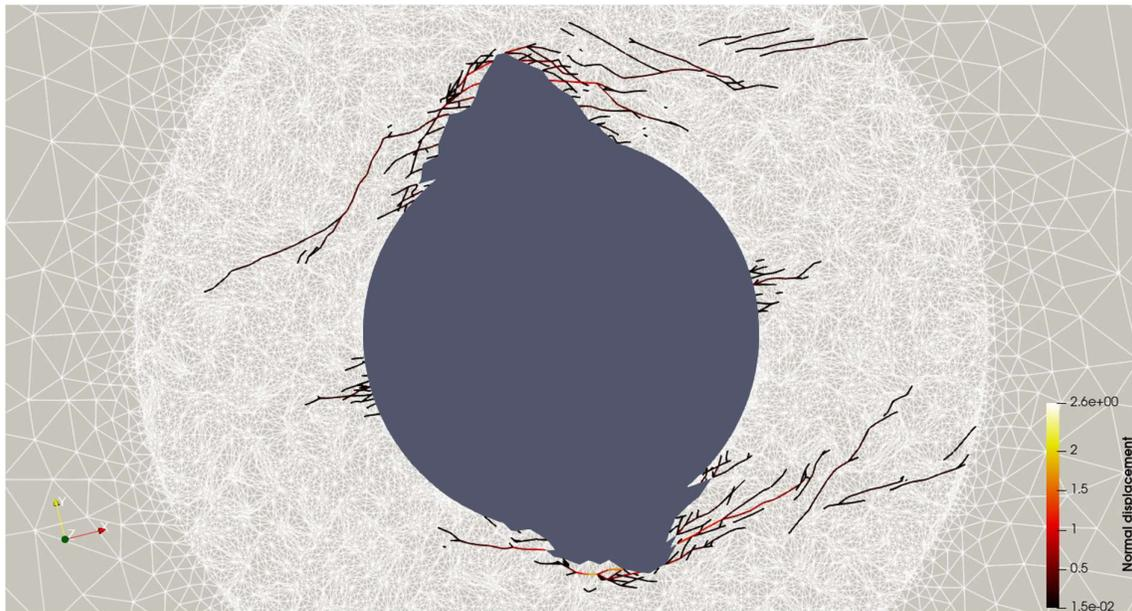
Fig. 4 Open cracks with normal relative displacements that exceed the established threshold value of 0.01 mm after the final excavation stage, are represented coloured.
