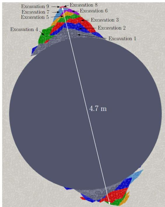
Fig. 3 Excavation process evolution and spalling depth for 2.35m.
