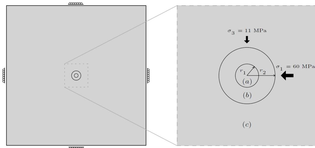
Fig. 1 Geometric domain of the Mine-by Experiment model, showing the detailed referenced zones and the initial stress conditions. Gravity effects are neglected, allowing the principal stresses to be aligned with the horizontal and vertical axes.
