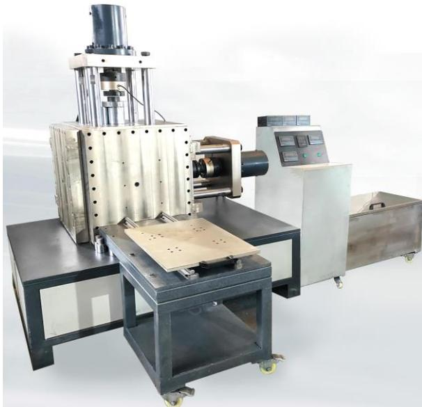
Fig. 2 Physical Test System for Multi-field Coupling Effects newly developed by Tsinghua University.
