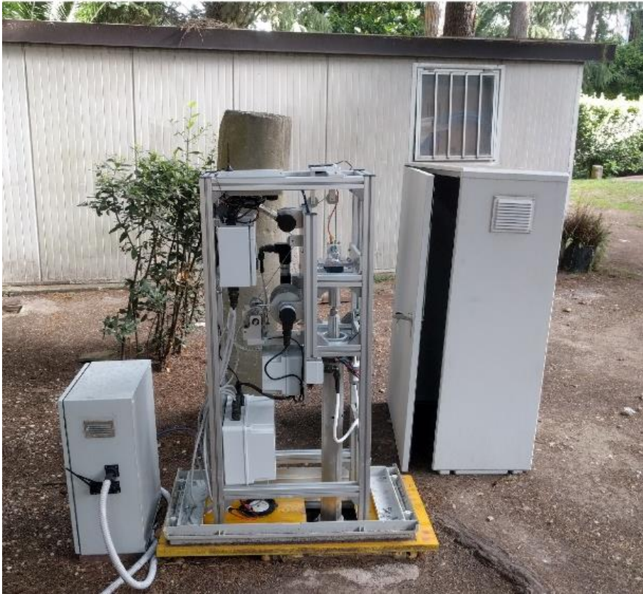
Fig. 2 Robotized inclinometric system without its protective casing
