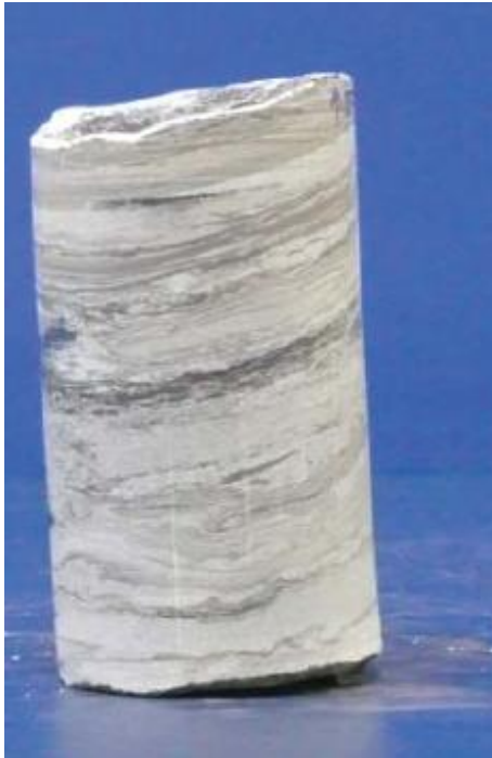
Fig. 2 Drill core from which specimens P13-A and P13-B were extracted (diameter 60mm).
