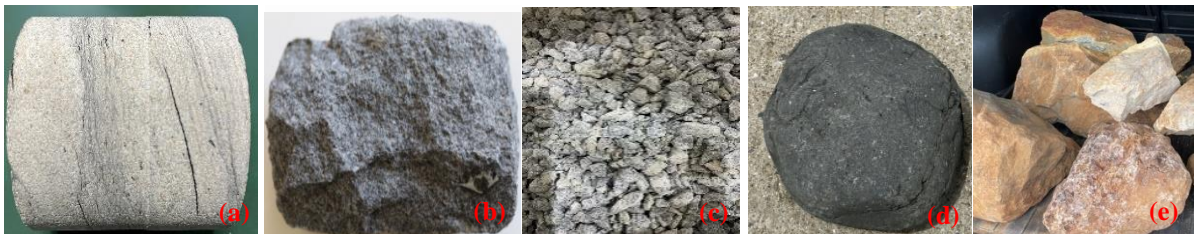
Fig. 2 Rock samples (a. Sandstone, b. Serpentinite, c. Peridotite, d. Basalt, e. Silicified andesite)
