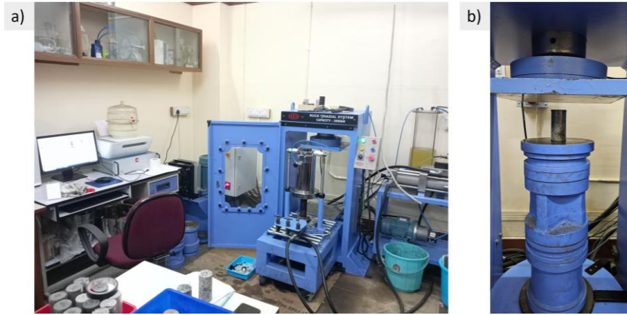
Fig. 3 Servo-controlled rock triaxial testing machine for a) triaxial compression and b) uniaxial compression tests.
