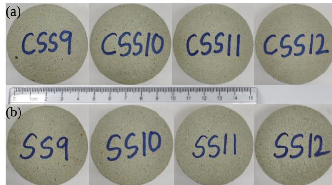
Fig. 3 Synthetic rock specimens used for (a) Dynamic compressive tests and (b) Dynamic indirect tensile tests.
