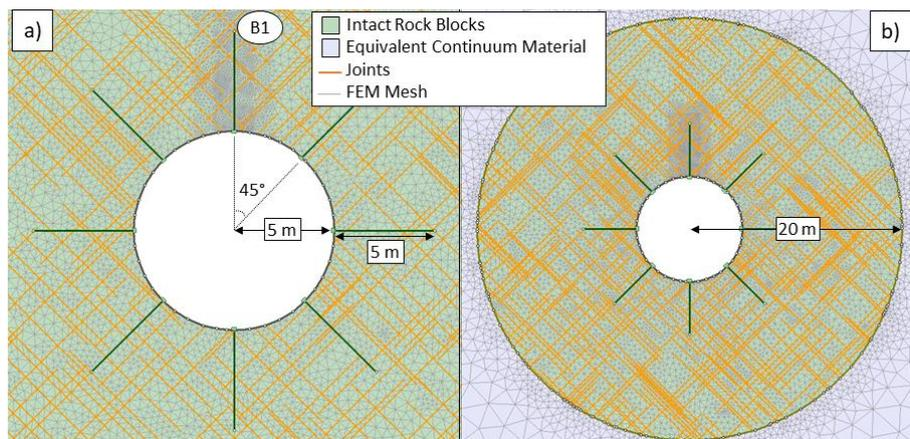
Fig. 7. a) Excavated tunnel in an explicitly modelled GSI 65 rockmass. “B1” indicates the bolt in the roof. b) Zoomed-out image of the explicit rockmass zone in the equivalent-continuum material, extending to pinned external boundaries.
