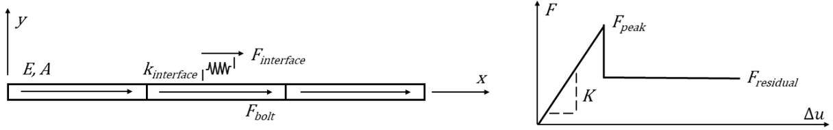
Fig. 2. Elasto-Plastic Interface bolt model discretization schematic and strength criterion, after Roescience (n.d.). The strength criterion schematic applies separately to both the bolt shaft and the bond interface.
