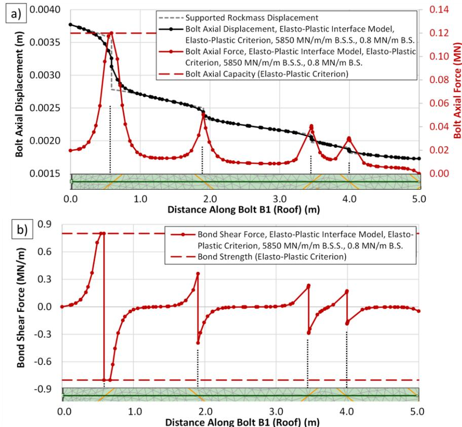
Fig. 8. a) Bolt axial displacement and bolt axial force and b) bond shear force for bolt B1 in the tunnel-scale model.
