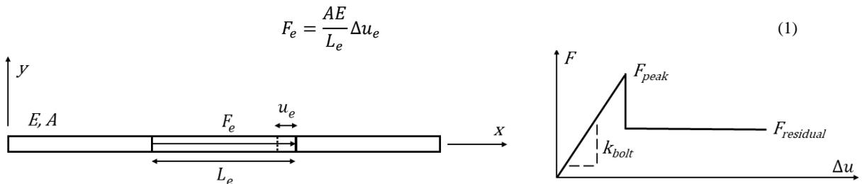
Fig. 1. Fully Bonded bolt model discretization schematic and strength criterion, after Rocscience (n.d.).
