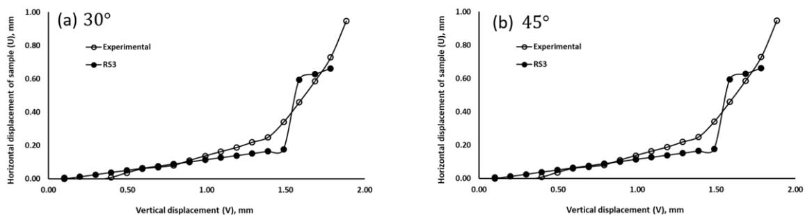
Fig. 7 Comparison of horizontal and vertical displacements of sample
