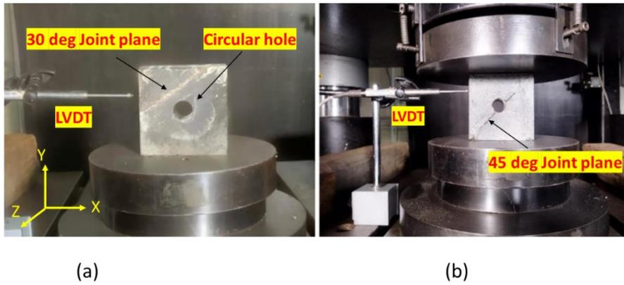
Fig. 1 Laboratory testing of sandstone samples (a) 30° joint and (b) 45° joint.
