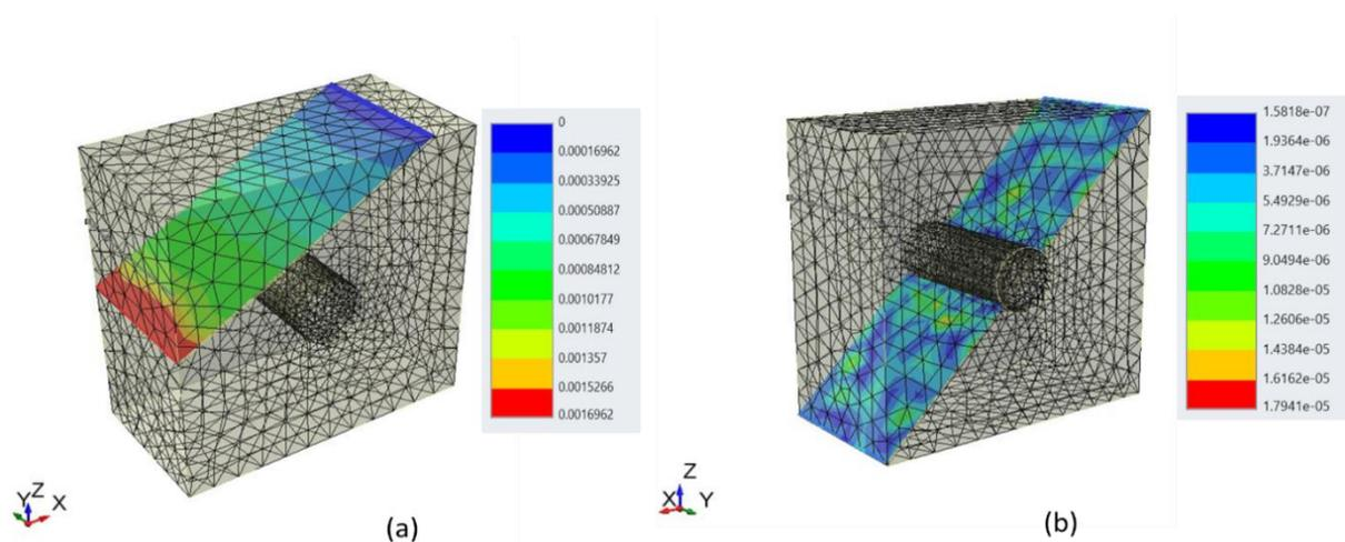
Fig. 8 Relative shear displacement (m) along joint (a) for 30° and (b) 45°
