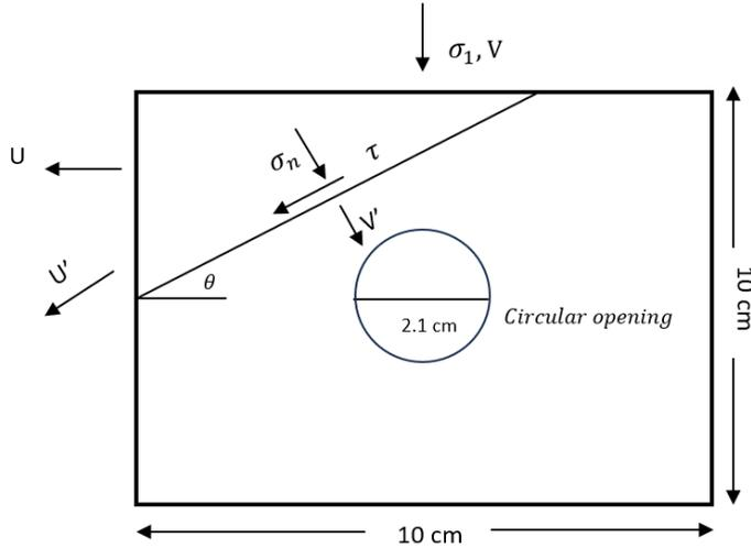
Fig. 3 Schematic diagram of applied stress and displacement on joint sample
