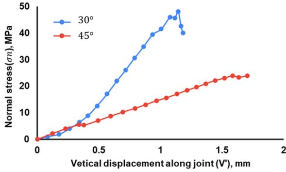
Fig. 5 Normal stress and vertical displacement
