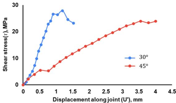
Fig. 4 Shear stress and displacement along joint
