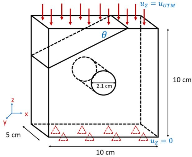
Fig. 6 Model dimension and boundary conditions
