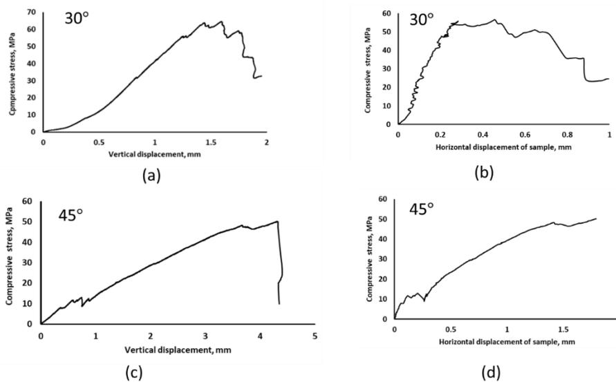
Fig. 2 Experimental plots of compressive stress versus vertical displacement and of compressive stress versus horizontal displacement of sample for 30° and 45°
