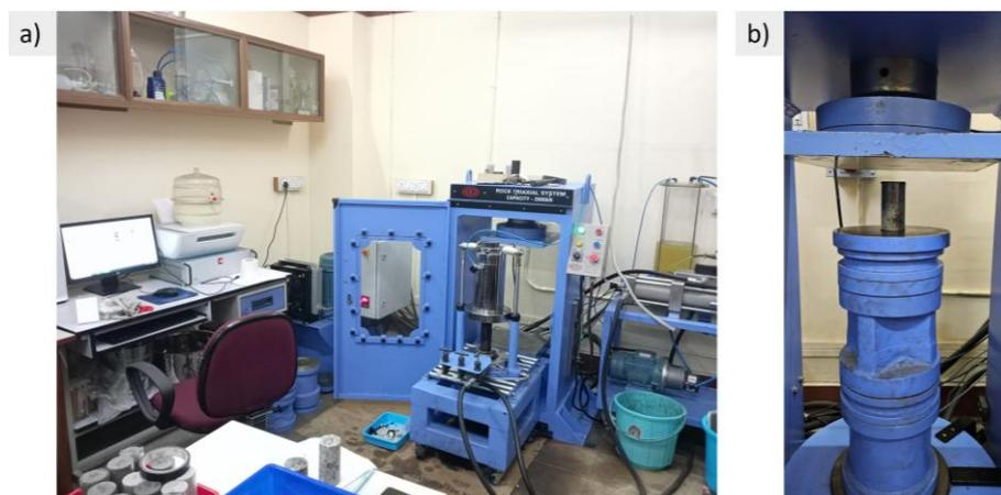
Fig. 2 Servo-controlled rock triaxial testing machine for a) triaxial compression and b) uniaxial compression tests.
