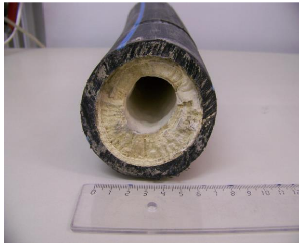
Fig.: Sinter formations in a drainage shaft inside the Gotthard Base Tunnel and heavily sintered pipe (Source: Harer)
