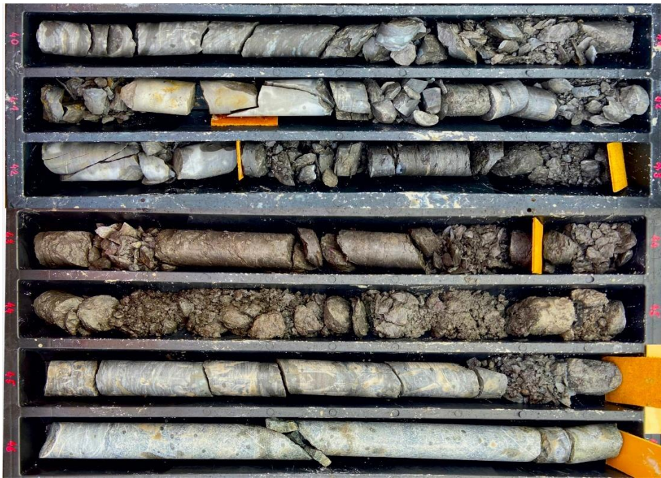
Figure 3: Encountering the Tachlovice overthrust in borehole J30, depth section 40–47 m. In the hanging wall of the fault zone are older shales and quartzites of the Kosov Formation (Ordovician), while younger shales and basalts of the Motol Formation (Silurian) were encountered in the footwall.
