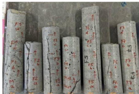
Figure 17: Drilled UHPFRC cores extracted from the tunnel lining
