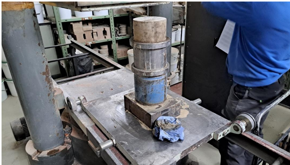
Figure 4: Arrangement of the Concrete Mixture Compression Test
