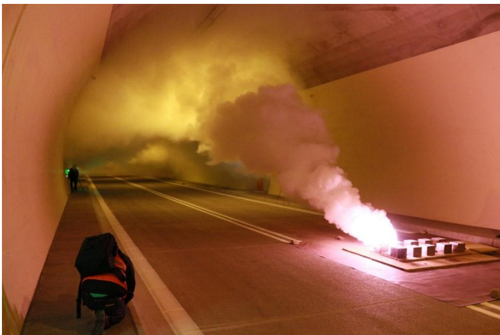
Figure 5: Experiment in situ (Poľana tunnel) with "cold smoke" – aerosol
