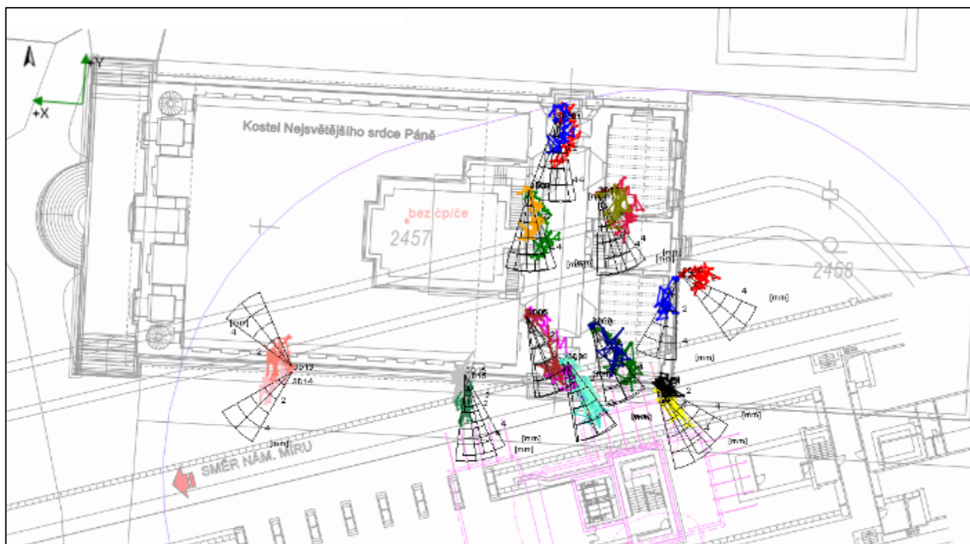
Figure 7: Fans showing the direction of deformation at positional points on the church facade (always two points above each other, inclination relative to the terrain)
