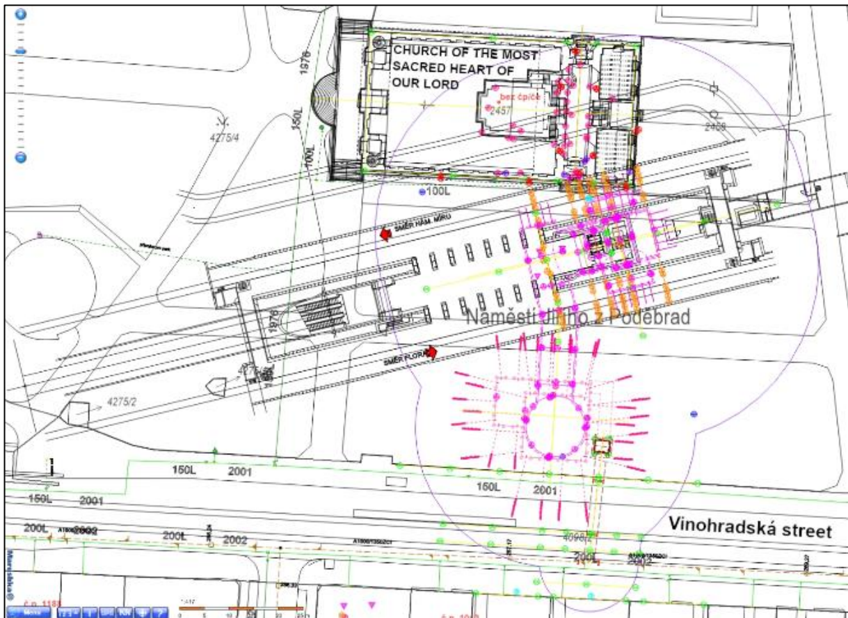
Figure 1: Distribution of measuring points from different methodologies and the zone of influence from the project documentation (see also the situation in (ČERMÁK, M., PAVELKOVÁ, B., MORÁVEK, R., 2014))
