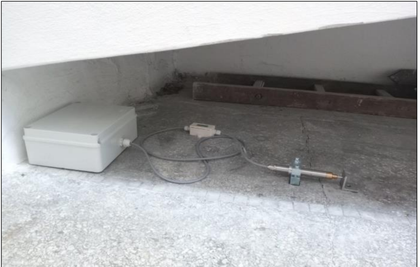
Figure 5: Automatic crack width measurement device with electronics for sending measured data to the geotechnical monitoring office (glued to the structure)
