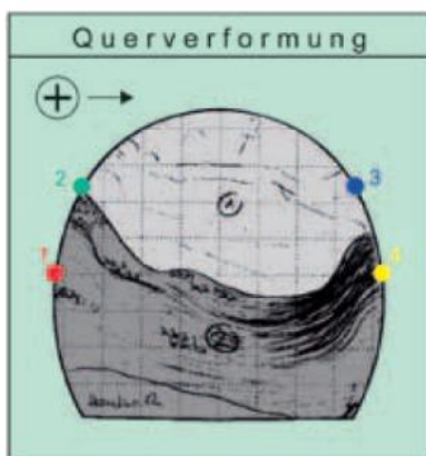
Figure 14: Geological face mapping with typical development of radial deformations (geodetic reflector measurements)
