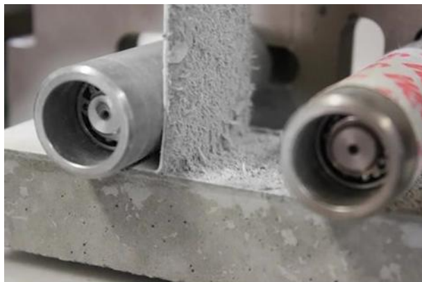
Figure 4: Strong bond between membrane and concrete
