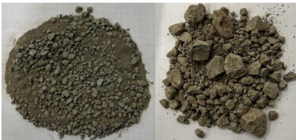
Figure 1: Clay samples used in the laboratory for the test campaign. DCC (left) e NCC (right). The difference in color is due to the different water content in the samples.
