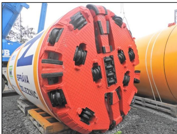
Figure 1: View of the cutting head of the bentonite shield.
