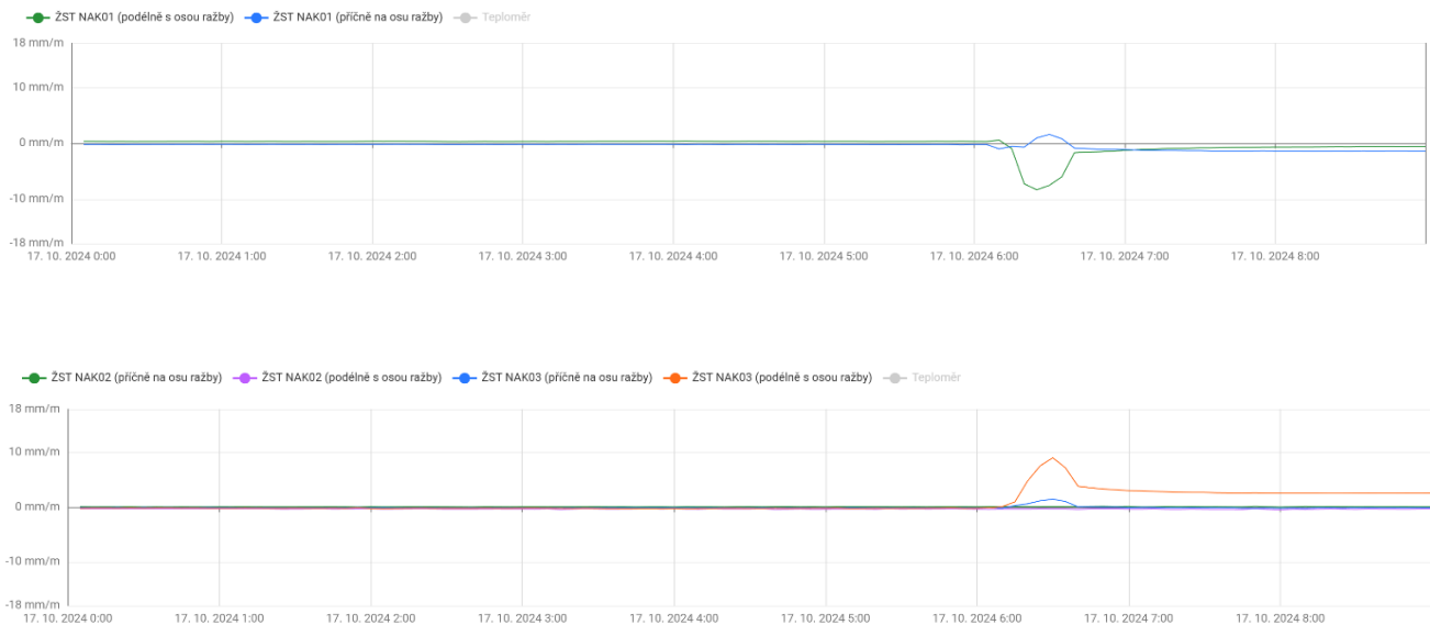
Figure 4: Graphical output from measurements taken by the tilt sensor on mast 268A.
