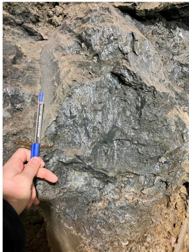
Figure 8: Slickensides in the face under clayey conditions (height of 45cm and a width of 30cm)
