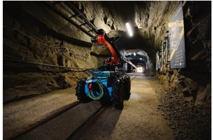
Figure 7 – JULBOT ver 1.0 – a robust machine designed for teaching, research, and development in the field of automated monitoring, not only of underground structures.
