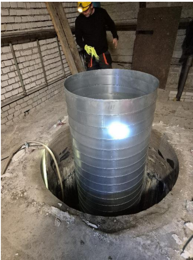
Figure 3: On the left is a large-profile underground drilling test for the MATEO project. The borehole has a diameter of 1650 mm and a depth of approximately 2000 mm. A pipe indicates the vertical storage of a container with spent nuclear fuel. On the right is a 3D conceptual design of the MATEO project experiment. Green narrow boreholes indicate rock monitoring. Dark gray indicates the concrete platform on the ground. Red indicates the heating element that will simulate the storage of spent nuclear fuel in a borehole with a diameter of 1650 mm and a depth of 5300 mm.
