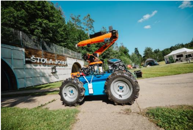
Figure 7 – JULBOT ver 1.0 – a robust machine designed for teaching, research, and development in the field of automated monitoring, not only of underground structures.
