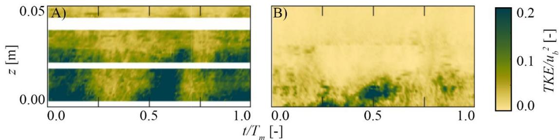
Fig. 2. Vertical and temporal distributions of the phase-averaged normalized turbulent kinetic energy  $TKE$  for an exemplary case for (A) the 2D model and (B) the 3D model.
