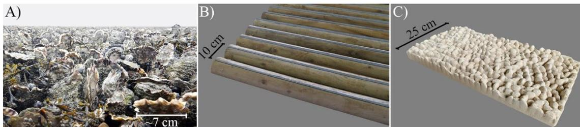
Fig. 1. Photographs of (A) an *M. gigas* reef, (B) the 2D model, and (C) the 3D surrogate model.
