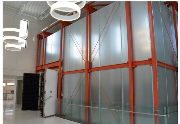
*AMS recently completed construction of a new \$1 million, 10,000 cubic foot electromagnetic compatibility (EMC) chamber for MIL-STD and IEC testing. It is designed to meet the EMC requirements of the NRC and EPRI and can accommodate equipment with weights up to 5000 lbs.*
