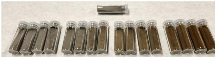
Figure 1: Powders following oxidation. Each group of 4 represents a temperature, increasing from 200°C (left) to 500°C (right). Within each group of four vials, times increase from left to right (i.e., 0.5, 1.0, 2.0, 4.0 hours). The single vial at the top is the virgin (unoxidized) powder.
