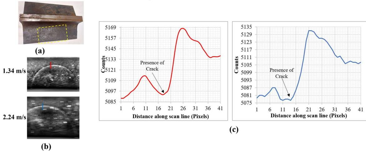
**Figure 4: S14 tested at 1.34 m/s and 2.24 m/s at 6000 W(a) S14 top view (b) IR images (c) Line ROI profiles**
