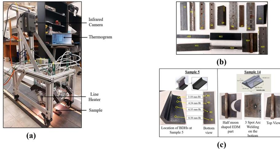
Figure 2: (a) IRIS setup (b) Tested samples with defects (c) Rail base samples
