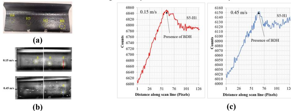
Figure 3: Sample 5 tested at 0.15 m/s and 0.45 m/s at 6000 W (a) S5 top view (b) IR images (c) Line ROI profiles
