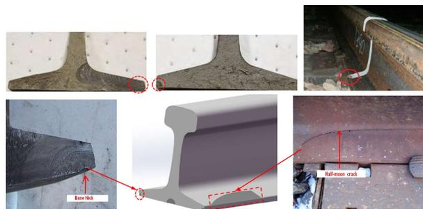
**Figure 1: Examples of various rail base defects seen in industry [1, 2]**
