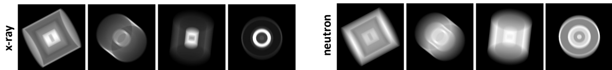
Figure 2: Example images comparing x-ray (left) and neutron (right) radiographs for the battery dataset.
