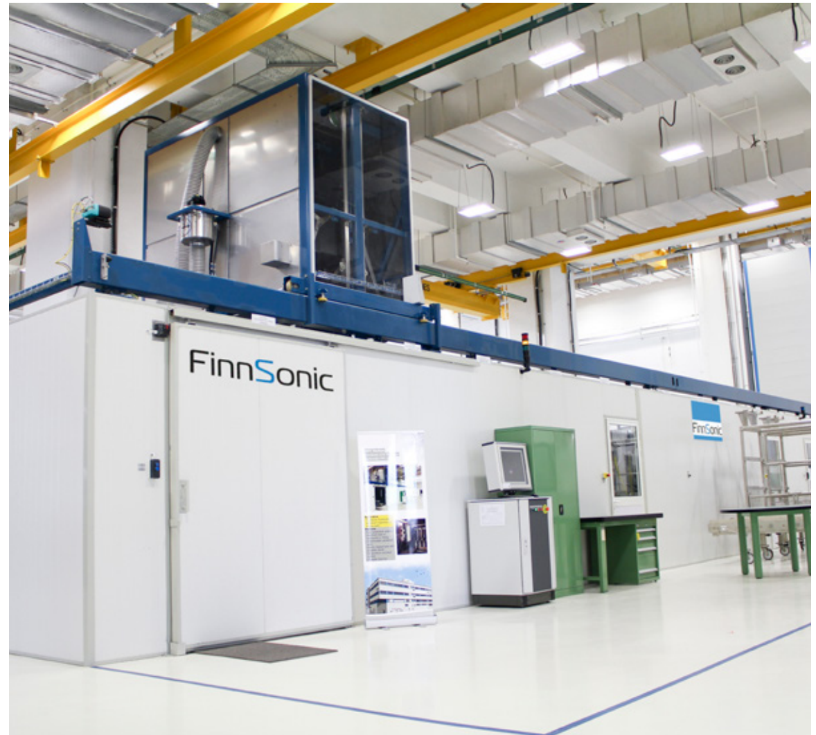
FinnSonic's automatic FPI line in Hong Kong, for inspecting jet engine parts. Line has been in use since 2010.
