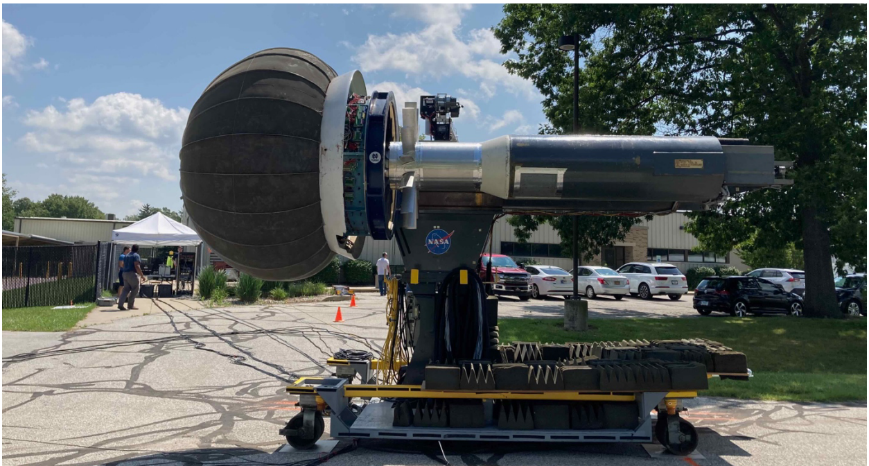
Figure 2. Advanced Noise Control Fan in Short Duct Configuration and Inflow Control Device.
