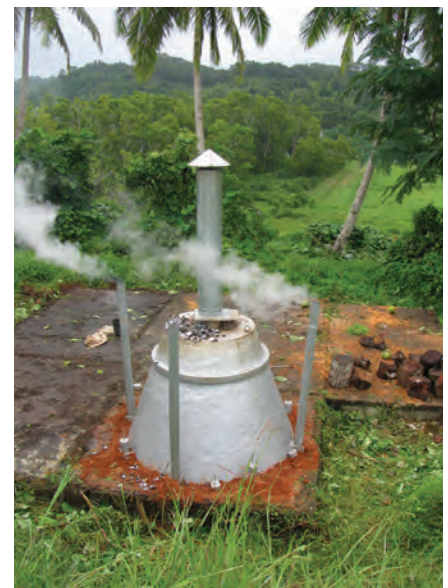
Biochar kiln in Naitasiri, Fiji: constructed by John Bennett from an old cement mix truck (Photo: Lex Thomson)
