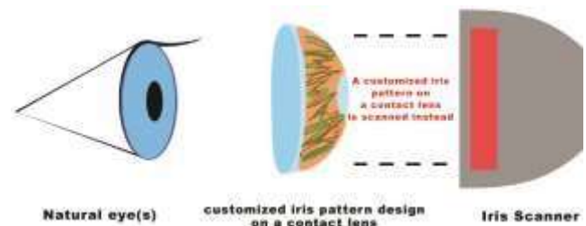
Figure 2. An idea about a wearable physical firewall in a form of contact lens ©Author
