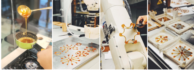
Figure 2 From left to right, the sequence includes simmering sugar syrup, employing a robotic arm to print patterns, lifting the sugar syrup design with a spatula, and finally, resin encapsulation. ©Shujiao.
