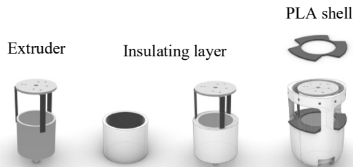
Figure 4 Design of the 3D printing extruder. ©Shujiao.
