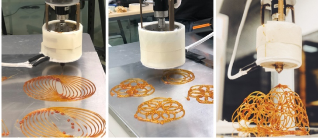
Figure 8 Printing test of parametric patterns. ©Shujiao.
